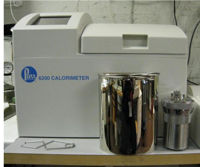
Reaction to fire tests for products - Determination of the gross heat of combustion (calorific value) (ISO 1716: 2018)
